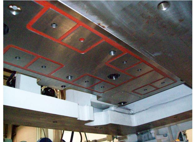
*Magnetic die clamping plate on inner slide of cupping press*
