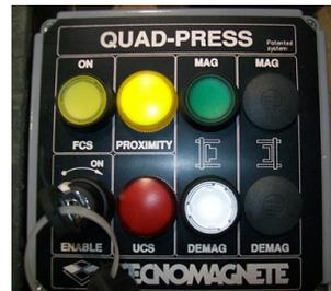
*Magnetic die clamping system control panel*
