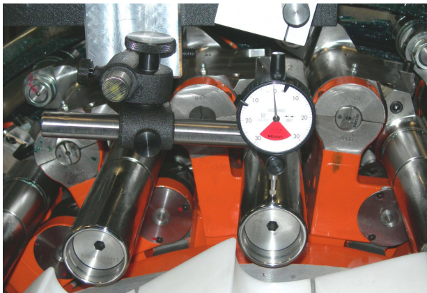
Concord Mandrel Circle Setting Fixture being used to set the mandrel circle
